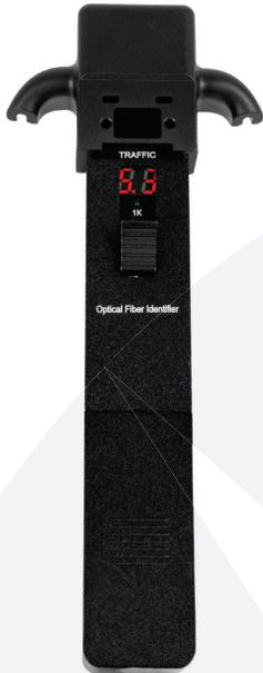
The OFI-30 Optical Fiber Identifier is a rugged, all-metal, easy-to-use installation and maintenance instrument, which can detect low frequency tones at 270Hz, 1kHz and 2kHz. When traffic is present on the fiber under test, an audible tone can be heard. Fiber traffic direction is indicated by sequential LEDs on the probe.
