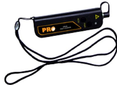
The VFL-5 is a compact but powerful visible light source with an output power up to 1mw. The VFL-5 can be used to locate sharp bends and breaks in jacketed or bare fiber. It can also be used to identify connectors in patch panels or identify fibers during splicing operations.
