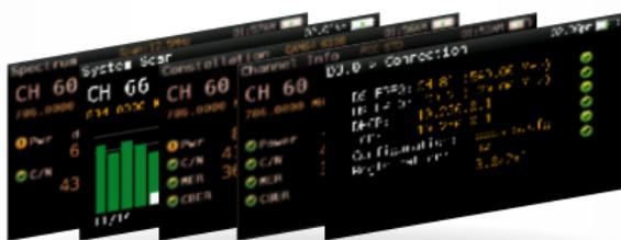
**Complete set of CATV features** such as Single Channel Measurements, System Scans, Tilt Function, Constellation, Spectrum Analyzer, Service Identification, Datalogs, Reverse Path Ingress Scan, Plan Learning... as well as **comprehensive DOCSIS 3.0 functionality** including Connection Status Information, Quality Parameters for every upstream/downstream carrier, Throughput and Modem Emulation.
