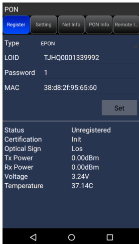
Figure 4: ONU registration info for a GPON/EPON system.
