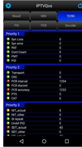
Figure 10: TR 101 290 status with color-coded test key.
