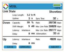
VDSL synch rates help the user determine if service can be maintained properly at the subscriber's location
