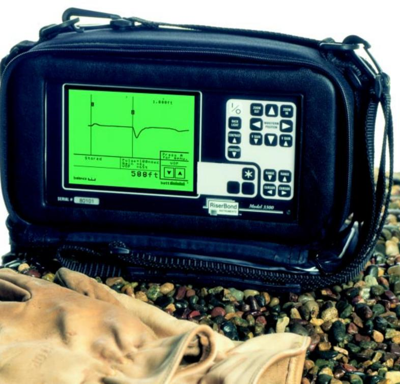
Use the exclusive SUPER-STORE waveform data storage to store both on-screen and off-screen cable waveform information. Move the cursors, change the VOP, and increase or decrease the vertical gain and horizontal zoom settings, *even on stored waveforms!*
