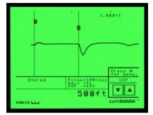
Selected functions and operations are controlled by the keypad, such as waveform position, horizontal zoom, vertical gain, cursors, range, contrast, and backlight. A popup menu is easily accessible for additional functions. Riser-Bond Instruments' unique popup menu system allows the operator to select and use a function while the waveform is active.
